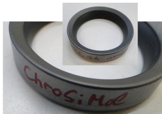
Figure 13: Internal combustion engine valve seat rings: replacement for Stellite armor
