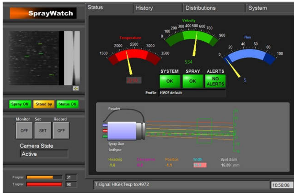
Figure 3: SprayWatch results showing droplet temperature and velocity at optimized spray parameters
