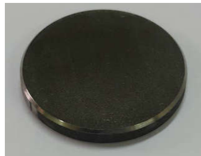
Figure 1: Sample extracted from the root of the turbine blade and the chamfer created on the sharp edge
