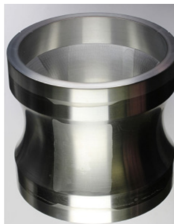
Figure 2: Hourglass shaped rotor made from NdFeB-Al composite and pure iron [5].
