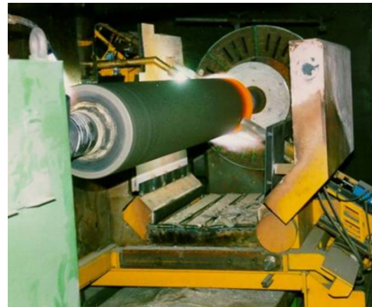
Figure 9: Fusing of Rolls with Self Fluxing NiCrBSiC alloys
