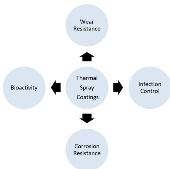
Figure 2: Applications of thermal spray coatings for orthopedic implants
