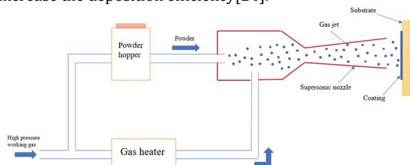
Figure 3: Schematic diagram of cold spray coating process
