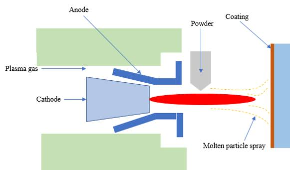
Figure 4: Schematic diagram of plasma spray coating process
