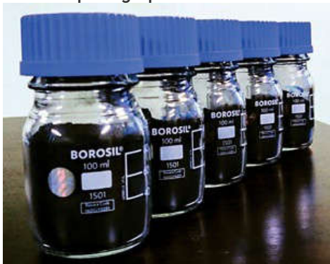
Figure 2: Graphite can be split into high-quality graphene (black powder in bottles) with a plasma spray technique used to make ceramic coatings (Credit: ACS Nano)
