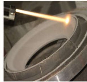
HARD SURFACING OF SEAT RING
