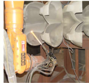
HARD SURFACING OF PELTON WHEEL
