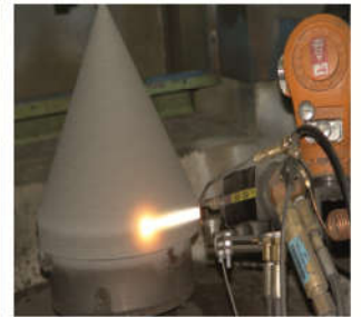
HARD SURFACING OF CONE
