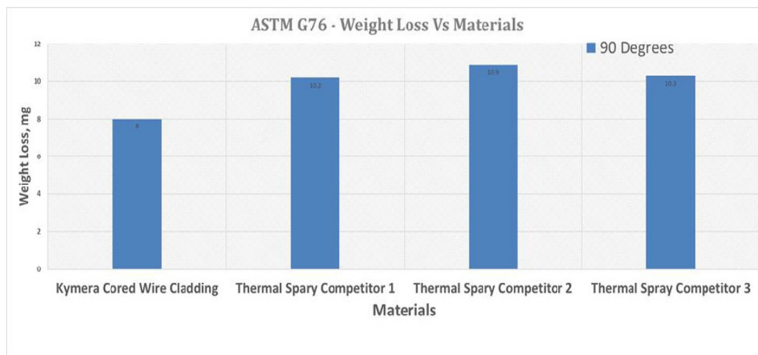
Figure 6: Relative erosion performance of tested thermal spray materials.
