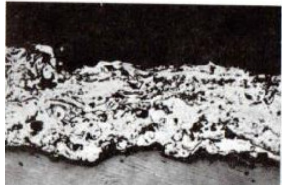
Figure 1: Zinc Sprayed Coating on Grit Blasted Steel
