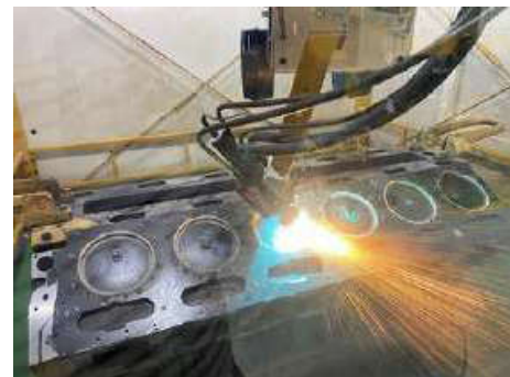
a: Arc Spray with Robotic Arm and 8400 Wire
