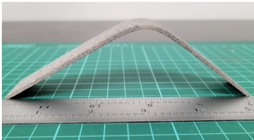
Figure 6: Post bend testing of Al base NbC composite coating
