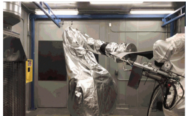
Figure 4: Cold Spray rebuilding of turbine Blade- GE [6]
