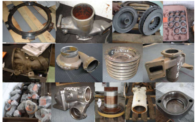
Figure 5: Another Parts of Engine and other Components that can be salvaged: +60.000 parts salvaged by Arc Spray at VMS.
