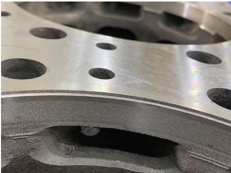
d: Machining to final Dimension in a Rottler EM104 or 105 Machine
