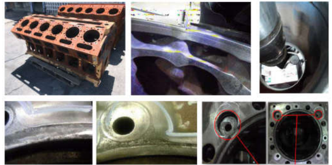
Figure 2: Main problems in engine blocks
