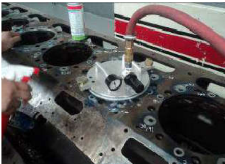
e: Perform the Leak Test
