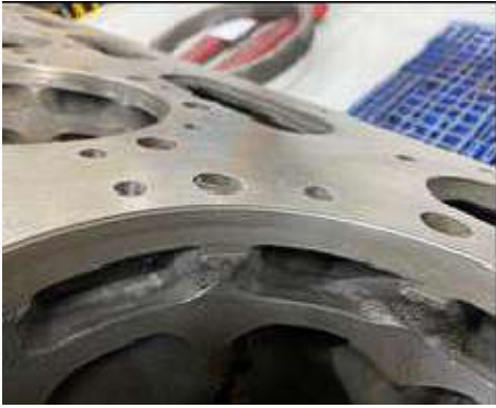
c: Machine D Shape for the Seal
