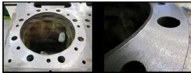
Figure 8: Dealers development 2017: fill up the water holes, liner seat and Surface. Using Smart Arc System + 8400 Wire, Optional 8293 Wire
