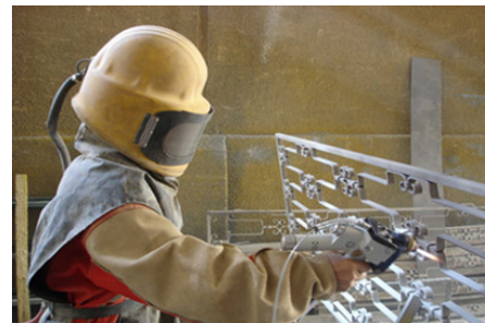
Figure 2: Protective and decorative metallization applied to a grid
